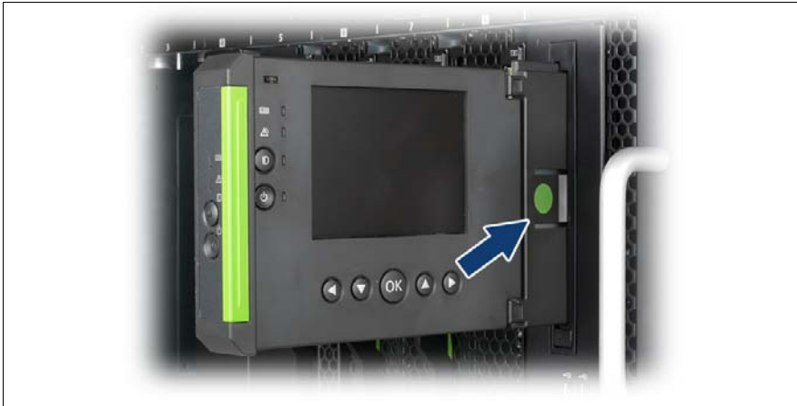
Figure 12: Locking the ServerView Local Service Display for Blade (rack version)
